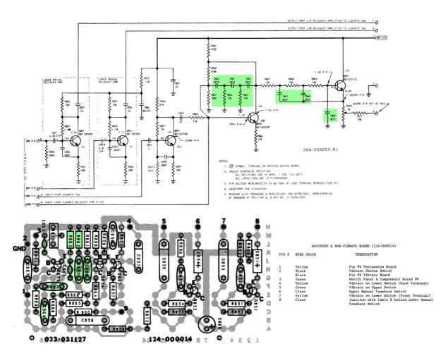
This is the original Hammond recovery transistor preamp board 124-000014, which is completely replaced by the MIG-T Preamp.
