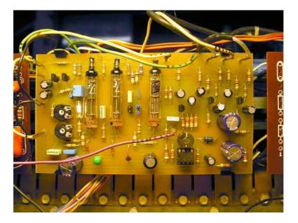
Upper picture above shows the pre-productional prototype of my **MIG-T** preamp. The tube in the middle of the PCB (type 1SH29b or 1J29b) is the **preamp output stage**, the two tubes to the left (type 1SH24b or 1J24b) work as the **additional overdrive stage**. The IC to the right is a LM2574ADJ "Simple Switcher", a high-efficiency switching power supply circuit which produces the 1,2V DC for heating. The transistorized preamp stages (upper right side) are
