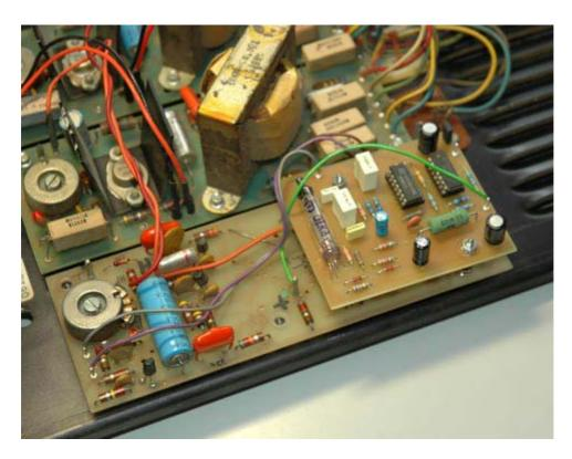
This is a MIG-LR affixed to a Leslie 760 amplifier panel. To the left you can see the Gain and Volume potentiometers. I have drilled them and glued a long M4 screw as an axle into the hole for easier access. The MIG-L board measures 80 x 65 mm; screw holes fit well above the crossover board so it can be mounted on top with two 6-32 UNC 1" screws and two 15 mm plastic spacers. Be careful not to short-circuit the MIG-L power plane with the screw/bolt.
