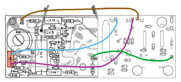
Wiring is very easy (only four wires), but some soldering necessary. C66 (marked red) has to be removed before inserting and soldering of input/output wires into circuit board holes. Be careful not to short-circuit the MIG-L power plane with the screw/bolt.
