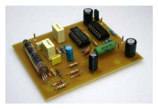
The MIG-L Leslie Tube Overdrive works with a real miniature tube. The MIG-LR even has a remote control input for switching between tube limiter and bypass mode.
